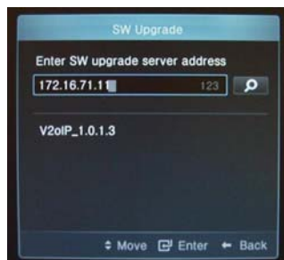
SW Upgrade window display - setting the TFTP server address and choosing the version
